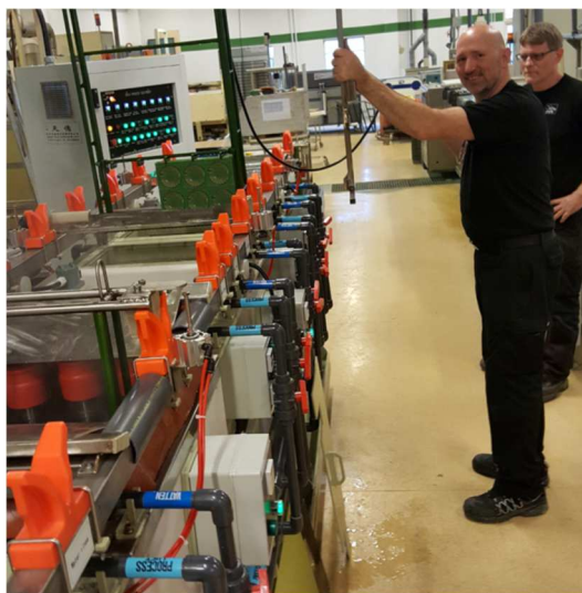
Per-Olof Javermark and Håkan Rask hoists the first panel with Gold in our new ENIG-process line.
