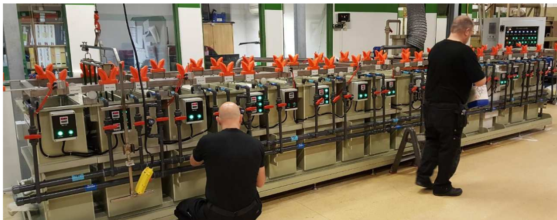
Per-Olof Javermark and Håkan Rask hoists the first panel with Gold in our new ENIG-process line.
